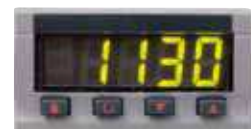
Over-temperature limit controller
